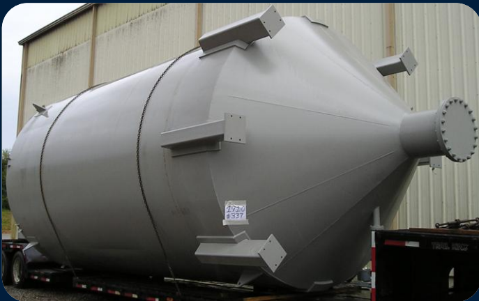
Job 1710: Suncoke- Pressurized Storage Bin (Bottom View)
