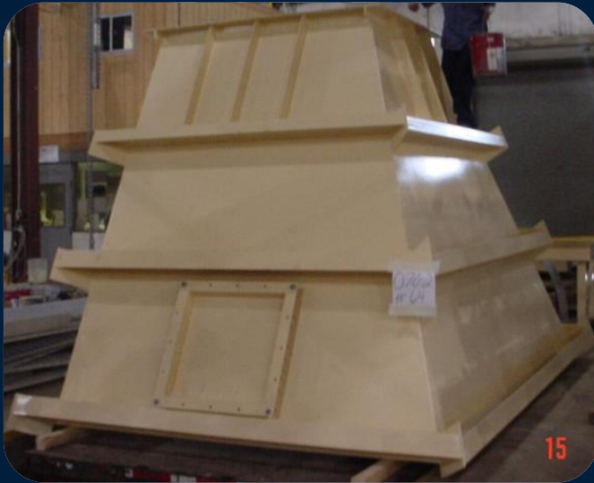
Job 0702: Xcel Energy (Commanche Station) - Surge Bin
