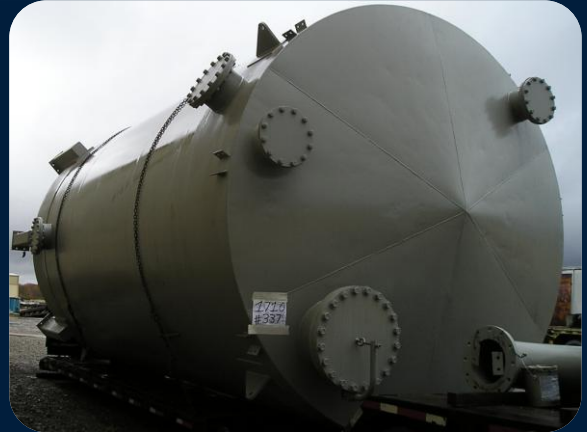
Job 1710: Suncoke- Pressurized Storage Bin (Top View)
